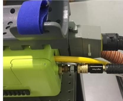
Universal mounting rails transform the handheld to over-the-shoulder or robot-mounted unit
